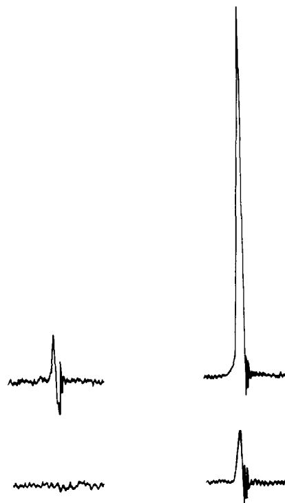
Figure 2. ^{19}\text{F} NMR spectra of acetonitrile solutions containing 0.2 M DMB and either 10^{-4} M (left) or 10^{-1} M TFA (right) in the dark (bottom) and during irradiation (top) with UV light. Splitting by the ortho-protons is not resolved in this dark spectrum but can be under higher resolution.
